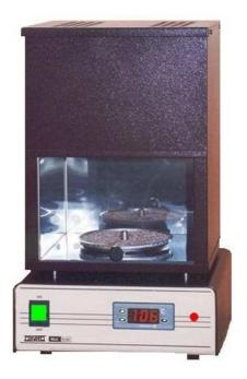
The control panel contains general switch, electronic temperature controller with digital indication and lamp synchronised
