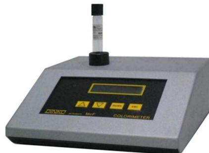
The Colorimeter has a range of 0 to 4 McFarland units. They are obtained readouts with a resolution of 0,01 McFarland in only 1 second and extrapolated readouts up to 10 McFarland Turbidity Units
