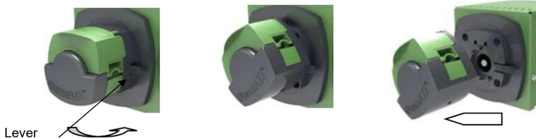
Offer the new head to the back plate at an angle that places the motor shaft to the shaft rotor inside the back plate at approximately 45°, facing the lugs on the housing.
