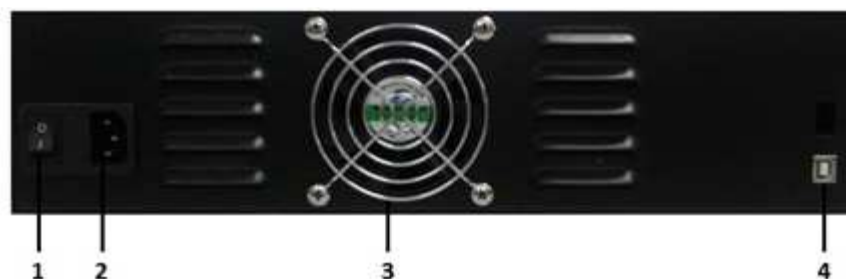
1--Power switch 2-- Power supply socket 3-- Cooling vent
