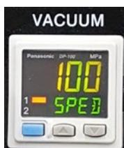
Press the **MODE** key, the controller gives us the option to change the color of the main display (see manual for options), by default as shown in the image.
