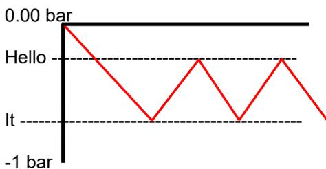
**Example** : to control the gap between 2 limits
