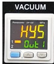
The working mode for our pump to control the vacuum between two points is this mode, **DO NOT MODIFY** .
