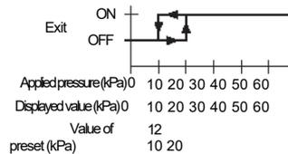
During remote zero adjustment. (Comparative outputs are in NA)
