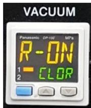
Press the **MODE** key, the controller gives us the option to change the units of measure. By default, the programmed unit is "Bars"
