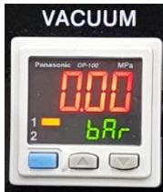
Keep the **MODE** key pressed for 2 seconds to enter programming.
